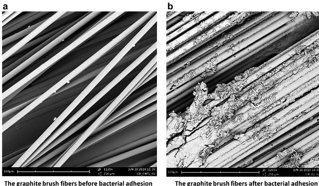
**Fig. 7 – The SEM pictures of graphite fiber brush (as anode in SCMFCs) before bacterial adhesion (a) and after bacterial adhesion (b).**
