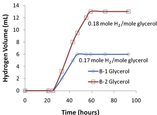
**Fig. 4 – The cumulative hydrogen production from purified glycerol (B1 and B2) from biodiesel waste stream in HPBs.**
