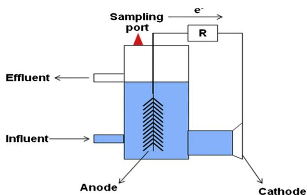
**Fig. 2 – The experimental setup of continuous mode SCMFCs.**
