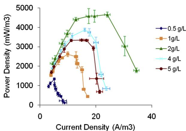
Fig. 5 – The variation of power density at different pure-glycerol concentrations in SCMFCs.
