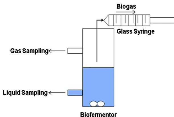
Fig. 1 – The experimental setup of batch mode HPBs.
