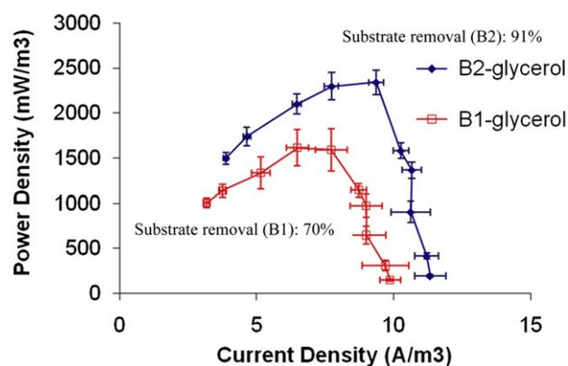
Fig. 6 – The power densities and current densities of SCMFCs utilizing the purified glycerol (B1 and B2) from biodiesel waste stream.
