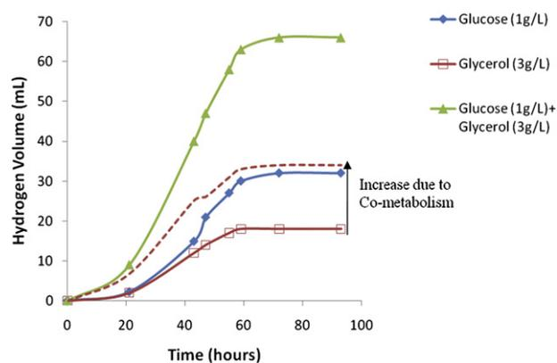
**Fig. 3 – The cumulative hydrogen production from pure-glycerol (3 g/L) and pure-glycerol-glucose co-metabolism (3 g/L glycerol with 1 g/L glucose) in HPBs.**
